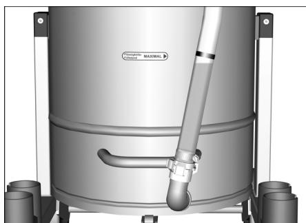
**Note:** The red marking on the drain hose shows the maximum admissible filling level.
